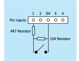
Note: For this feature to work correctly it is essential to connect the resistor at the contact end of the loop and not the dialler end. The Monitoring Centre must also enable the monitoring of this facility on the dialler within the IRIS Secure Apps receiving system.
