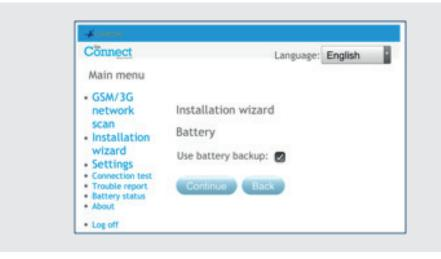
Once Installation Wizard is completed and any additional panel interface configuration setup via the settings menu, check/configure the panel for the connection method being used and the current battery status.
