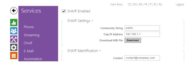
The **2N Helios IP** intercoms integrate a remote intercom supervision functionality via the SNMP. The integrated SNMP agent becomes available when the **Enhanced Integration** licence key is added. The intercoms support the SNMP version 2c.
