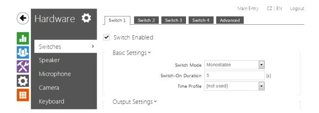
Switches provide a very flexible and efficient control of such intercom peripherals as electric door locks, lighting, additional ringing signalling, and so on. **2N Helios IP** allo ws you to configure up to 4 (depending on model types) independent all-purpose switches.
