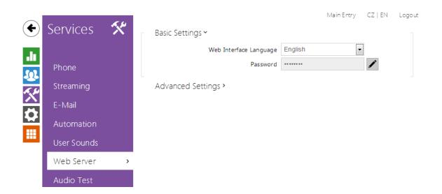
You can configure your **2N Helios IP** intercom using a standard browser which accesses the integrated web server. Use the secured HTTPS protocol for communication between the browser and intercom. Having accessed the intercom, enter the login name and password. The default login name and password are **admin** a nd **2n** respectively. We recommend you to change the default password as soon as possible.
