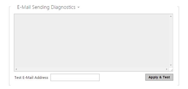
Click **Apply & Test** to send a testing e-mail to the defined address with the aim to test the functionality of the current e-mail sending setting. Enter the destination e-mail address into the Test e-mail address field and press the button. The current e-mail sending state is continuously displayed in the window for you to detect an e-mail setting problem if any on the intercom or another network element.
