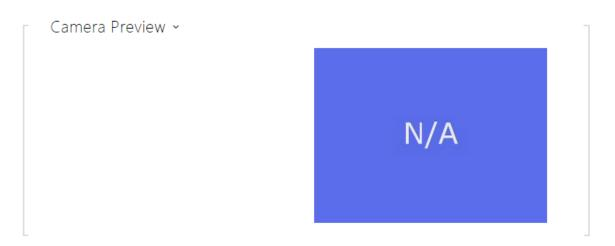
The Camera Preview window displays the current image received from an external camera. If the external camera is disconnected or configured incorrectly, the N/A characters are displayed on a blue background.
