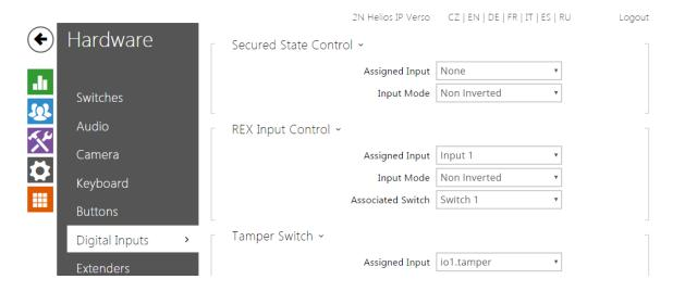
In this configuration section set the parameters associated with digital inputs and their interconnections with other intercom functions. The digital inputs are available in selected intercom models or where appropriate equipment is installed (Vario/Force model card readers, e.g.).
