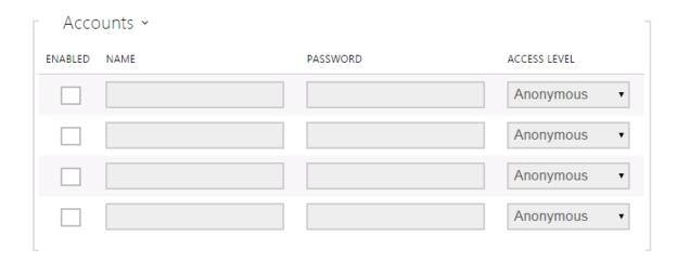
For full ONVIF functionality it is required to set at least one user account and set proper access right, according to ONVIF specification and used VMS. Without this, only basic
