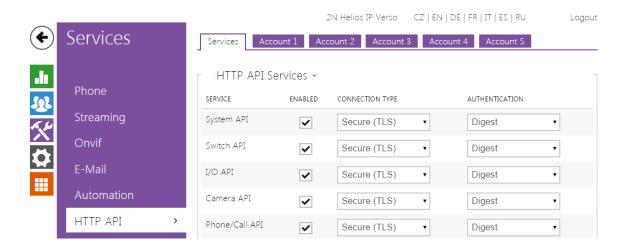
**HTTP API** is an application interface designed for control of selected **2N Helios IP** functions via the **HTTP**. It enables **2N Helios IP** intercoms to be integrated easily with third party products, such as home automation, security and monitoring systems, etc.
