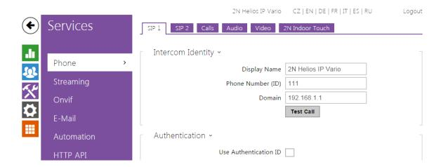
The Phone service is one of the basic functions of the intercom: helps you establish connections with other IP network terminal equipment. The **2N Helios IP** intercoms support the extended SIP and are compatible with and certified by the leading SIP PBX and terminal equipment manufacturers (CISCO, Avaya, Broadsoft, etc.).
