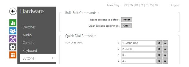
Assign the **Directory** / **Users** users to the quick dial buttons. By default, all available intercom buttons are assigned to the listed users. A non-assigned button can be used for automation or switch activation, for example.
