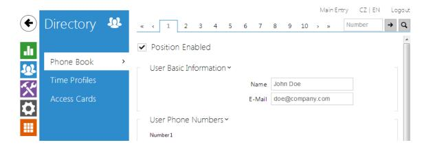
The Users list is one of the crucial parts of the intercom configuration. It contains user information relevant for such intercom functions as quick dialling, RFID card/code door unlocking, missed call e-mails and so on.
