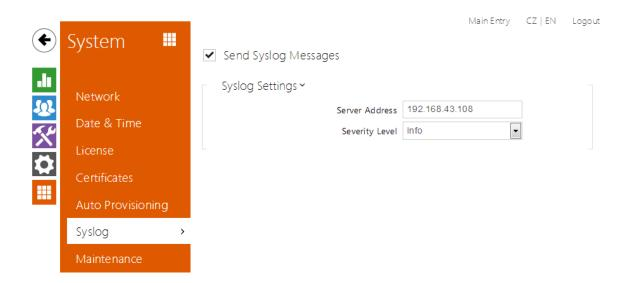
The **2N Helios IP** intercoms allow you to send system messages to the Syslog server including relevant information on the device states and processes for recording, analysis and audit. It is unnecessary to configure this service for common intercom operation.
