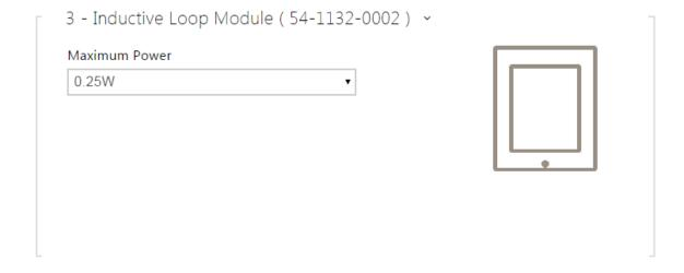
■ **Maximum power** - set the maximum transmission power for the induction loop antenna. A higher transmission power means a wider range, but less power for other intercom functions. The convenient default value is 0.25 W under normal circumstances.
