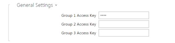
■ Access key – set the access key to be shared by the intercom and 2N® Indoor Touch. If the access keys do not match in the intercom and 2N® Indoor Touch, the intercom cannot call the 2N® Indoor Touch device and the 2N® Indoor Touch device cannot receive video from the intercom. Each intercom can be assigned up to three access keys and thus become a member of up to three independent 2N® Indoor Touch groups.
