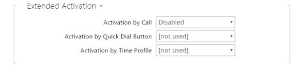
• Activation by call – enable switch activation by an incoming or outgoing call, for example. During an outgoing call the switch is activated after SIP message 180 Ringing is received. The called party confirms ringing by this message. The switch is active during the whole call in the bistable mode, and activated by the
