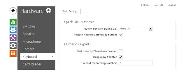
This configuration section helps you set the numeric keypad and quick dial button functions. **2N Helios IP** allows you to:
