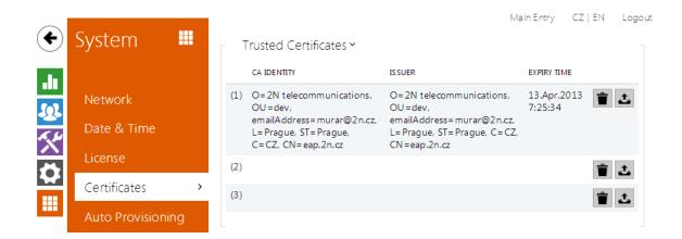
Some **2N Helios IP** network services use the Transaction Layer Security (TLS) protocol for communication with other LAN devices to prevent third parties from monitoring and/or modifying the communication contents. Unilateral or bilateral authentication based on certificates and private keys is needed for establishing connections via TLS.
