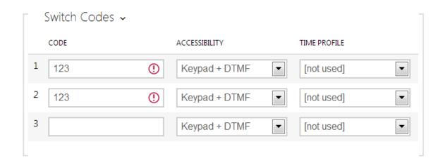
The table above includes a list of universal codes that help you activate switches from the phone or intercom keypad. Up to 10 universal codes can be defined for each switch (depending on the particular intercom model).
