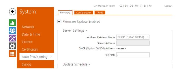
The **2N Helios IP** intercoms help you update firmware and configuration manually, or automatically from a storage on a TFTP/HTTP server selected by you according to predefined rules.
