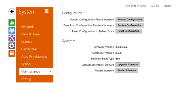
Use this menu to maintain your intercom configuration and firmware. You can back up and reset all parameters, update firmware and/or reset default settings here.
