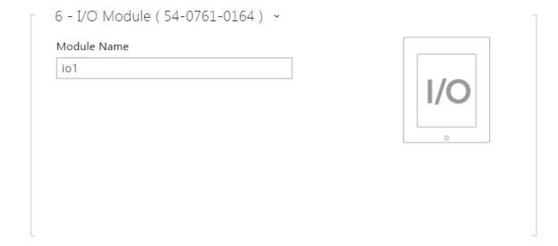
■ **Module name** – set the module name for input/output specification in the SetOutput, GetInput and InputChanged objects in **Automation**.
