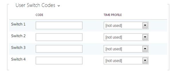
Each user can be assigned a private switch activation code. The user switch codes can be arbitrarily combined with the universal switch codes defined in the **Hardware | Switches** menu. If the codes are identical with the codes already defined in the intercom configuration, the mark will appear at the colliding codes.
