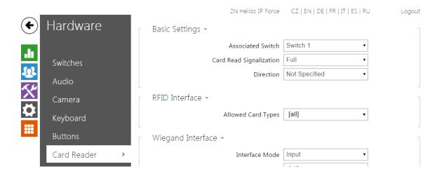
This menu is available in the  $2N^{\otimes}$  Helios IP Vario and  $2N^{\otimes}$  Helios IP Force models only. Configure the  $2N^{\otimes}$  Helios IP Verso card reader in the Extenders menu.
