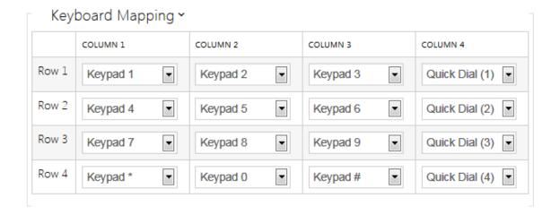
You can assign one function to each matrix position: numeric keypad keys 0 through 9, \*, # or one of the quick dial buttons 1–16.
