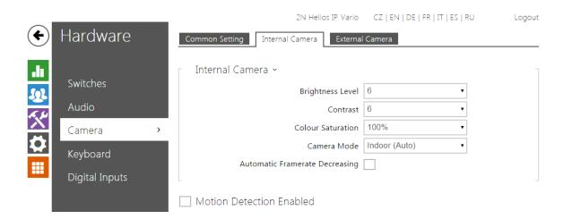
This menu is only available in the **2N Helios IP** models that are equipped with an internal camera or can be connected to an external camera. The camera signal can be streamed directly into the call via a videophone, sent by E-mail, streamed via ONVIF/RTSP to another device (a video surveillance device, e.g.), or simply HTTP downloaded from the intercom in the JPEG format.
