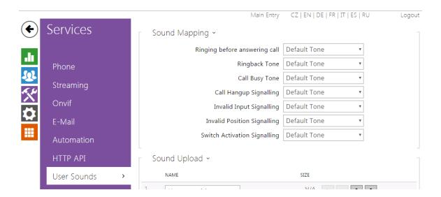
The **2N Helios IP** intercoms provide standard signalling of operational statuses by tone sequences; refer to the Signalling of Operational Statuses subsection. If you find the standard sound signalling inconvenient, modify the sounds for the following statuses:
