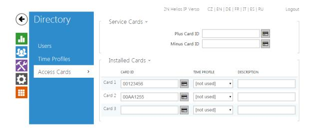
Each intercom user can be assigned one or more access RFID cards. Typically, the card ID is included in the users list together with such user data as phone numbers, E-mail address and so on. Or, you can define the RFID cards in the Installed Cards list, which defines a limited number of unassigned cards reserved for visitors, for example.
