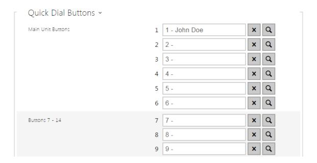
Display the list of all potentially available intercom buttons including those that are physically absent. In some intercom models ( $2N^{\otimes}$  Helios IP Vario,  $2N^{\otimes}$  Helios IP Verso), the button list is divided into 8/5-item groups corresponding to the button
