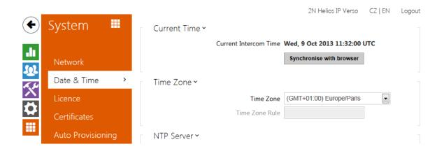
If you control validity of phone numbers, lock activation codes and similar by time profiles, make sure that the intercom internal date and time are set correctly.
