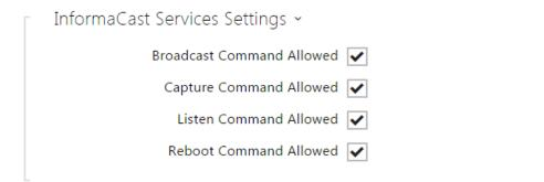
**Broadcast enabled** - enable the Broadcast command to set up an audio stream sent from the Informacast server to the intercom.
