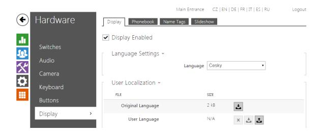
Some **2N**<sup>®</sup> **Helios IP Vario** models are equipped with a colour LCD display. The device state is displayed (call progress, door opening, etc.) and the following modes are available:
