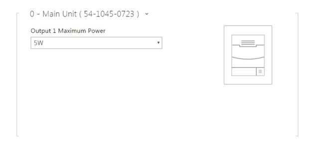
Output 1 maximum power - set the maximum load to be connected to the power output available on the basic unit. When the output is active, the consumption of the other modules (backlight level, etc.) can be adjusted automatically in order that the maximum allowed consumption of the intercom cannot be exceeded.
