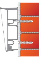
Wall (surface) mounting is used where flush mounting is inapplicable (in concrete and steel structures, entry barrier columns, etc.). The frame is not used.
