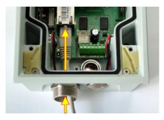
6. Move the sealing including the cover along the cable as far as the bushing body, or add a plug if necessary.
