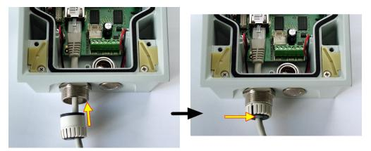
7. Replace and tighten the nut.
