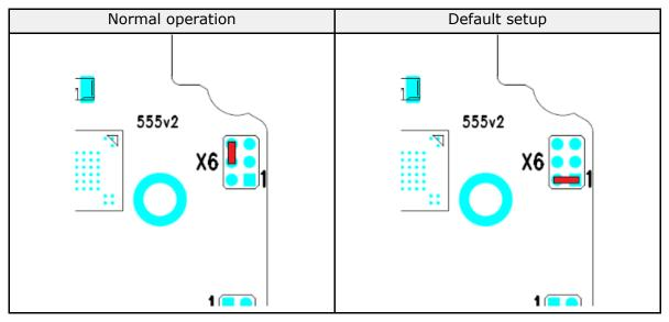
Figure: Configuration jumpers X6, PCB version 555v2
