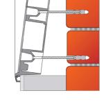
Cut out the thermal insulation layer using the template (the same as for classic brick wall).
