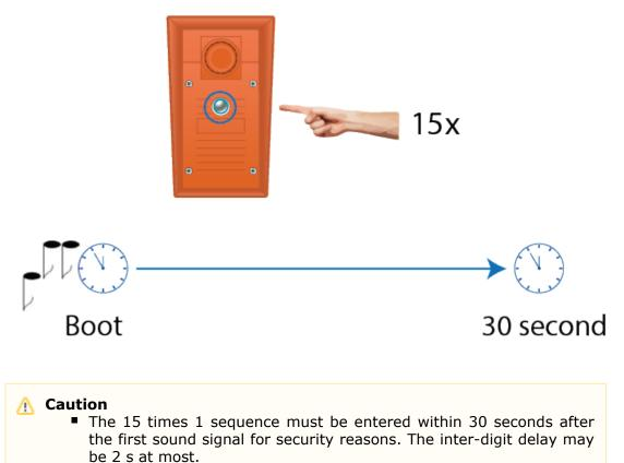
The static IP address mode will be switched into the dynamic IP address mode and vice versa upon restart.
