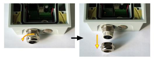
2. Remove the sealing including the cover from the bushing. Cut either of the components as shown in the figures.
