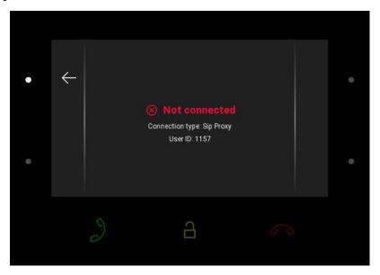
The My2N/SIP Proxy section displays the current state of the My2N/SIP Proxy connections.
