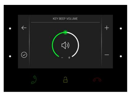
Press the right-hand upper/lower button to increase/decrease the key beep volume. Press the left-hand lower button to confirm the key beep volume level selected. The change will not be saved unless confirmed.
