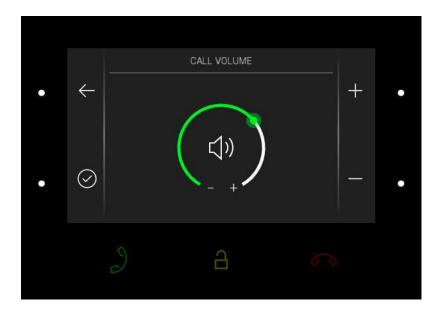
Press the right-hand upper/lower button to increase/decrease the call volume. Press the left-hand lower button to confirm the call volume level selected. The change will not be saved unless confirmed.
