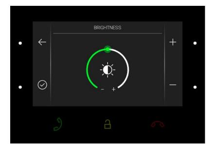
Press the right-hand upper/lower button to increase/decrease the display brightness. Press the left-hand lower button to confirm the brightness level selected. The change will not be saved unless confirmed.
