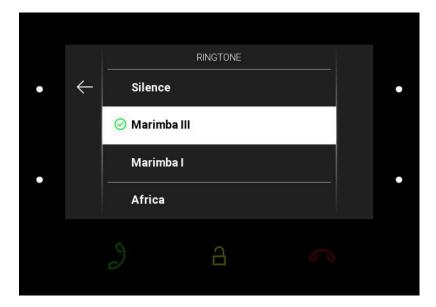
Press the right-hand upper/lower button to move up/down the ringtone list. Press the left-hand lower button to confirm the ringtone selected. The change will not be saved unless confirmed.
