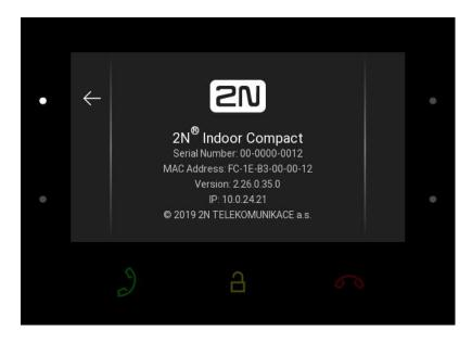
This section provides basic information on the device (serial number, MAC address, FVW version, IP address).
