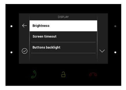
Press the right-hand lower button at the icon  $\bigcirc$  to display the Display section. Here set the display brightness, idle timeout and button backlight.
