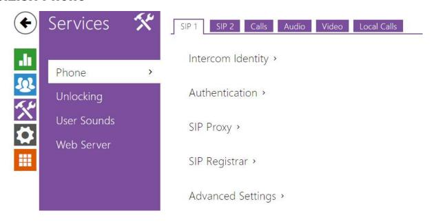
Phone is the basic function of  $2N^{\mathbb{R}}$  Indoor Compact allowing you to establish connections with other IP network terminals.  $2N^{\mathbb{R}}$  Indoor Compact supports the extended SIP.
