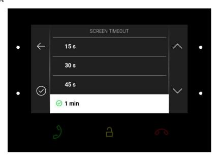
Set the maximum idle time (i.e. when the user does not control the device) after which the sleep mode is switched on automatically. Press the right-hand upper/lower button to move up/down the time value list. The change will not be saved unless confirmed.
