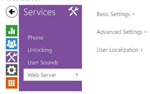
2N® Indoor Compact can be configured using a common browser that approaches the web server integrated in the device. The HTTPS protocol is used for the browser - device communication. Enter the login user name and password first. The default values are admin and 2n respectively. We recommend to you change the default password as soon as possible.
