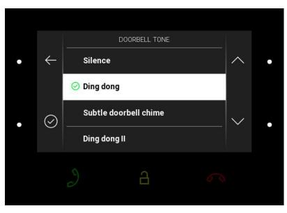
Press the right-hand upper/lower button to move up/down the doorbell ringtone list. Press the left-hand lower button to confirm the ringtone selected. The change will not be saved unless confirmed.
