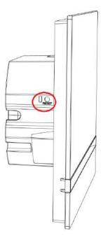
To **restart the device** press the Reset button on the device backside. The restart will be performed within 10 seconds, during which the device keeps shining and fails to respond to other key presses.
