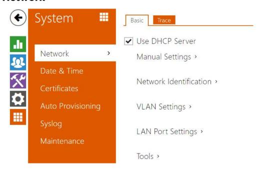
To be connected to the LAN properly, **2N** \*\*Indoor Compact has to be assigned a valid IP address or obtain the IP address from the LAN DCHP server. The Network section helps you configure the IP address and DHCP.
