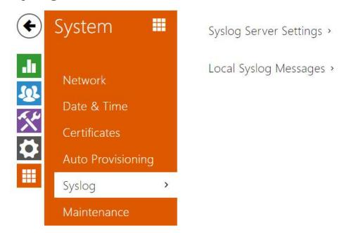
**2N** \*\*Indoor Compact allows you to send syslog messages including relevant device state and process information to a syslog server for recording and further analysis or auditing of the device observed. It is unnecessary to configure this service for common operations.
