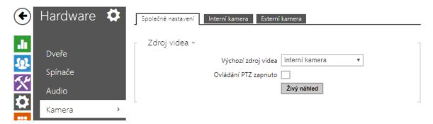
This menu is only available in the **2N LTE intercom** models that are equipped with an internal camera or can be connected to an external camera. The camera signal can be streamed directly into the call via a videophone, sent by E-mail, streamed via ONVIF /RTSP to another device (a video surveillance device, e.g.), or simply HTTP downloaded from the intercom in the JPEG format.
