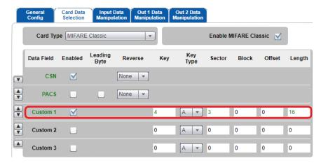
**Note:** CSN is set to show only for demonstration purposes, and is not necessary for reading custom data.
