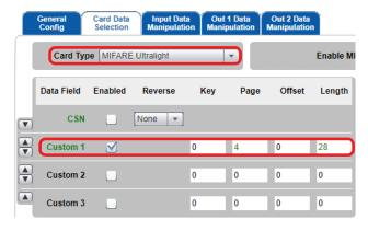
**Note:** Although Ultralight pages are only 4 bytes long, you can specify any length, as the reader will read subsequent pages until it has enough bytes.
