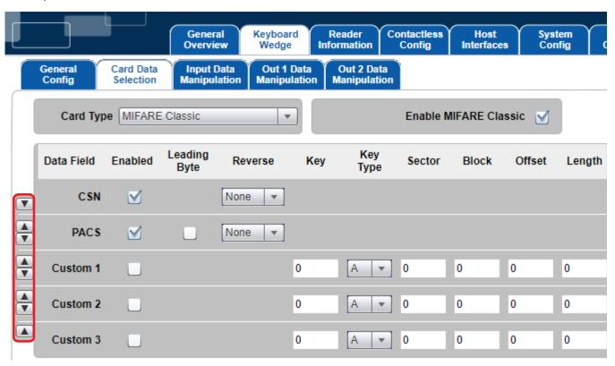
Separate data fields from each other by using pre- and post-strokes (Out2 Data Manipulation tab).
