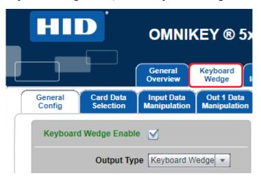
Keyboard wedge operation is a highly configurable read-only application of the reader. Care should be taken to configure the product correctly, and to enable only the card technologies and data that are needed at each installation, to lower the likelihood and/or prevent rogue credentials from being introduced to the application.
