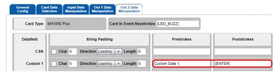
This allows all data from block 3 to be read from the card, and produces the following output:
