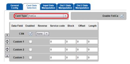
3. Select the **Out 1 Data Manipulation** tab. To see the FeliCa IDm (CSN), select HEX/DEC/ASCII depending on the required output:
