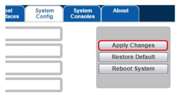
**Note:** The **Reboot System** button is only necessary when changing operational modes (CCID, Keyboard Wedge, Custom Report) so the reader can re-enumerate with the host system as the proper device, and when changing configuration parameters under the Host Interface tab (Changing Ethernet Settings, Enabling UART, etc.). Click **Reboot System** only after clicking **Apply Changes.**
