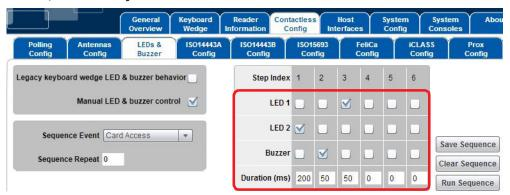
**Note:** Always ensure that you end the card access sequence with the beginning state of the USB Ready Sequence, to ensure a smooth transaction, and that the colors are reset to the USB Ready state as shown above. This will prevent an unwanted buzzer/LED state remaining after the sequence has completed. See *Section 5.1.3.1: Incorrect LED/buzzer sequence*.
