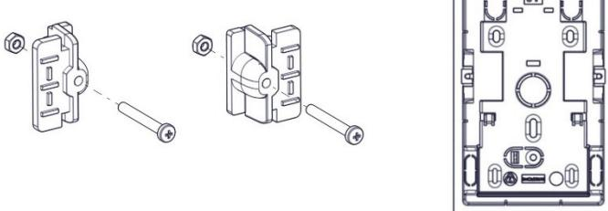
**2.** Using the mounting template, take measurements for drilling a hole in the wall.
