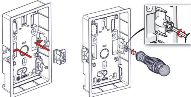
Insert a screw in each tab and attach a nut to the end of each screw. Position the two tabs in their slots and secure the two screws as shown
