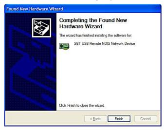
⇒ The USB RNDIS Driver should now be installed on the host PC.
