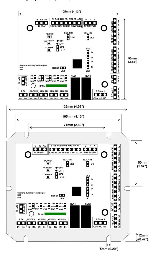
The following diagram displays the location of the ports on the ADD5100:
