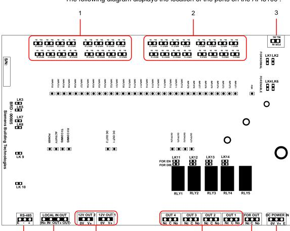
The following diagram displays the location of the ports on the AFI5100:
