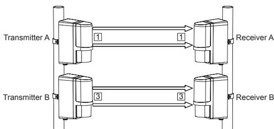
Since Receiver B may receive the infrared beam from Transmitter A, select their frequencies as shown in the figure above. (In the figure, each number in the square indicate a channel numbers.)
