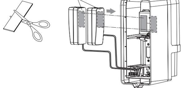
6 Run the cables so that they are not pinched between the chassis and back box.
