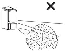
Do not install the receiver in a location where it is exposed to direct sunlight.
