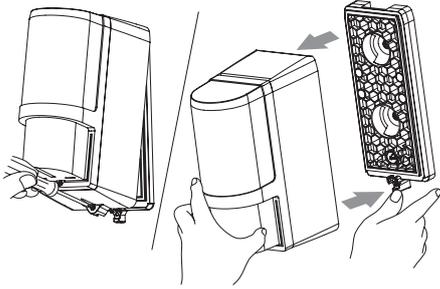
2 Fix the chassis to the wall.
