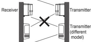
Install the unit more than 1 m (3.3 ft.) away from the wall or fence that are running parallel to the beam.
