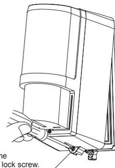
Tighten the back box lock screw.
