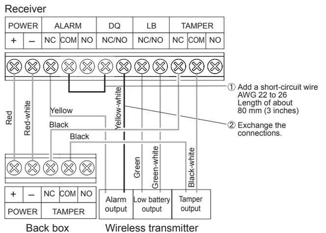
Wiring example when Using N.C. Transmitters
