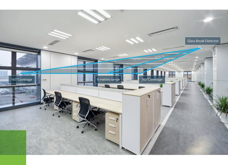
The AGB800-AM, has the same solid foundation of the AGB800, with the added functionality of anti-mask. At the time of writing the AGB800-AM is the only acoustic glass break detector to pass the rigorous requirements of EN50131-2-7-1:2013, Grade 3 for high security installations. The AGB800-AM anti-mask functions provides unique tamper protection, which is signaled via a separate relay.
