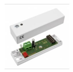
CD 475 offers reliable monitoring against attacks with mechanical tools. The CD 475 is a chock- and vibration detector with 3 separate detection channels: an integration channel / saw channel for weak signals with long duration, a counting channel that senses strong impact on the monitored surface and an explosion channel which senses very strong signals from e.g. an explosion.
