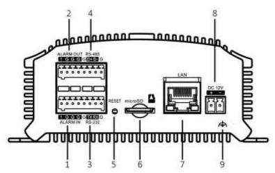
The rear panel of DS-6704HUHI provides 4 alarm in and 2 alarm out interfaces.
