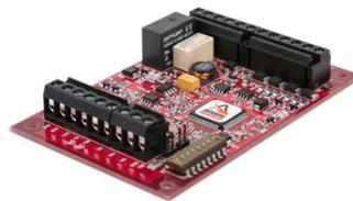
The Mercury Security AC-MER-CONT-MR50 Series 3 from Avigilon is an enhanced, high performance, reliable single card reader interface panel that offers all the I/O needed
