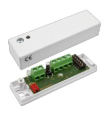
CD 470 offers reliable monitoring against attacks with me-chanical tools. The CD 470 is a chock- and vibration detector with 3 separate detection channels: an integration channel / saw channel for weak signals with long duration, a counting channel that senses strong impact on the mon-itored surface and an explosion channel which senses very strong signals from e.g. an explosion.
