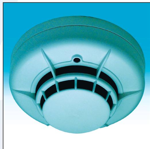
The HRZ-1005T detector also has an integral LED, which illuminates to provide a local alarm signal. This latches on, and remains illuminated until the detector is reset by a momentary power interruption. An optional remote LED annunciator may be used to repeat any alarm signal.
