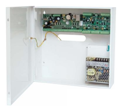
Access control kit for four doors. The kit consists of metal enclosure with power supply, networked access controller and IO expander. The controlled doors can be managed on both, read-in and read-out side, by RS485 (MCT series readers). In case the RACS CLK/DTA (PRT series readers) or Wiegand readers are used, doors can be
