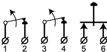
MC 447 is a surface mount magnetic contact with double NC function and 6 screw terminals. It can be used in both alarm and access control systems for monitoring e.g. doors and windows against unauthorised opening.
