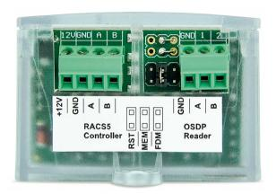
The interface enables the connection of a reader that uses OSDP protocol to the MC16 series access controller (RACS 5 system). The interface works as a communication converter from the OSDP v2 protocol to the RS485 EPSO 3 (Roger) data transmission standard.
