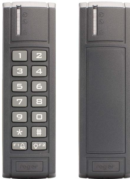
MCT12E series reader is outdoor identification terminal designed for use in the RACS 5 access control system. It enables identification of users by means of EM 125 kHz cards. Communication with the controller is carried out via a modified RS485 standard, which allows star
