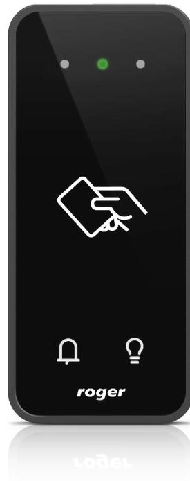
The MCT80M-BLE is an access terminal dedicated to RACS 5 access control and building automation system. Terminal enables identification of users by 13.56 MHz MIFARE<sup>®</sup> Ultralight/Classic/DESFire/PLUS cards and by use of smartphone with NFC or Bluetooth technology. In case of Bluetooth identification the reading range can reach up to 10 meters while other methods offer few centimetres of reading range. The mobile identification requires Roger Mobile Key application installed on
