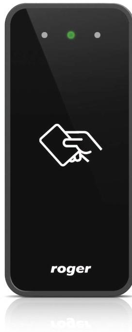
The MCT80M is an access terminal dedicated to RACS 5 access control and building automation system. Terminal enables identification of users by means of 13.56 MHz MIFARE Ultralight<sup>®</sup> and MIFARE<sup>®</sup> Classic cards. MCT80M is equipped with RS485 interface which is used for communication with access controller. Be-
