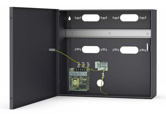
The ME-40-24V enclosure is dedicated to RACS 5 modules and devices which require installation on DIN rail along with 17 Ah battery. The enclosure is equipped with single DIN rail, DC power supply 24 V/2.2 A and tamper contact and mains fuse switch. Access to the internal space of
