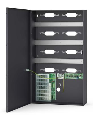
The ME-44-S enclosure is dedicated to RACS 5 modules and devices which require installation on DIN rail along with 17 Ah battery. The enclosure is equipped with 3 DIN rails, buffered power supply 13.8 V/10 A, tamper contact and main fuse switch. Access to the internal space of
