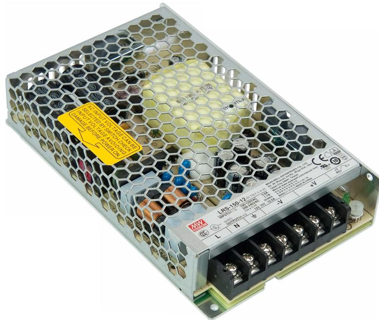
PS8D is LRS-150-12 (Mean Well) power supply unit with rated output voltage increased from 12.0 V to 13.8 V by means of original output potentiometer. PS8D is dedicated to installation in RACS 5 system, particularly to supply MCX2D and MCX4D expanders and PSD4D power distributors but it can also be used for other applications if its nominal conditions of use are satisfied. The PSU is
