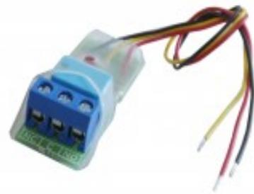
The RC 1 is a very compact and universal relay card with alternating (NC/ NO) relay function. Connection of the relay is provided via screw terminal with wire protection. Control signal and supply is connected via 15 cm cable. Transistor control of the relay means a very low control signal is required (1 mA). An activated relay is indicated via a LED. On the back of the device there is a self-adhesive pad for ease of installation.
