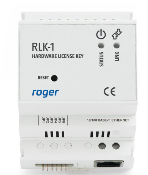
RLK-1 is a hardware license key connected to the computer network on which the licensed software runs. Communication with RLK-1 is encrypted using AES128b
