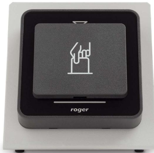
RUD-4-DES is a desktop reader and writer for MIFARE® Classic, Plus (S, X) and DESFire (EV1, EV2) cards which also allows reading an EM 125 kHz standard proximity cards. It is supplied directly from a USB serial port, which is also used for communication with the PC. The device has a stable metal desktop stand with a card holder. The RUD-4-DES can be used as a card enrol reader for the access control system or any other application which requires a card reader. A card can be enrolled straight
