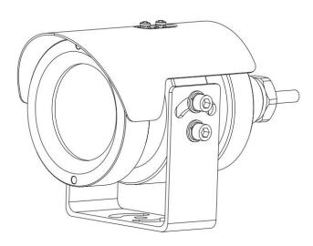
Step 3 Fix the wall-mounted bracket on the wall with four expansion bolts. See Figure 3-6. Figure 3-6 Fixing the wall-mounted bracket on the wall
