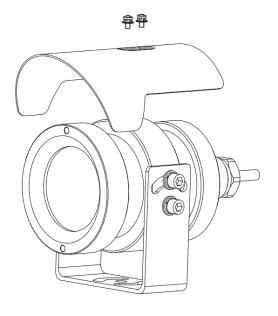
Step 2 Secure the sunshield on the camera with two M3\*6 screws. See Figure 3-5. Figure 3-5 Securing the sunshield on the camera
