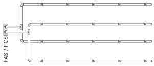
Pipe configurations for dual detector dependency
