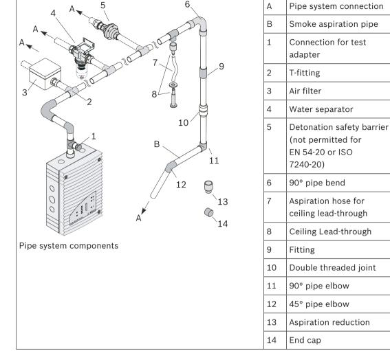
During planning/design, a distinction is drawn between area monitoring and equipment monitoring. For both applications, PVC pipes and halogen-free pipes can be used but the restrictions of EN 54.20 must be observed. The pipes used for equipment monitoring should be halogen-free.
