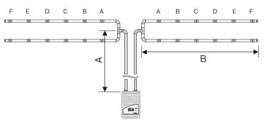
Example of a pipe system with long pipe feed lines for area monitoring
