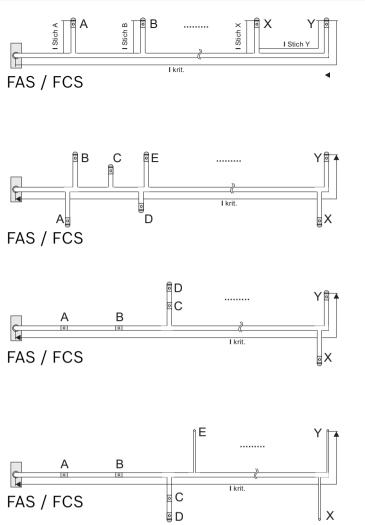
The branch pipes must be projected in accordance to the figure (project planning with branch pipes). The project planning of I-pipe described in the figure must be copied to every single sampling branch of other pipe forms (U, M, double-U pipe system).
