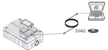
Figure 3.4: FAS-ASD-DIAG Diagnostic SoftwareDiagnostic software for importing and reading out the device data
