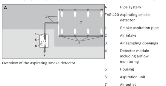
To guarantee reliable operation even under the most difficult conditions (clean rooms, recycling area), there are numerous accessories available, such as air filters, water separators and detonation safety barriers.
