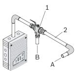
Components of manual blowing-out systems
