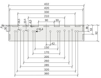
Figure 5.3: Bore distances with mounting type MT-1
