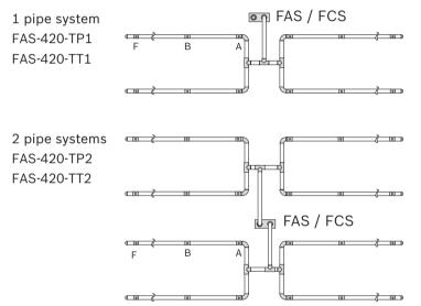
Double U-pipe system for space protection
