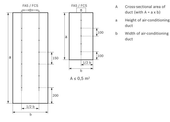
A > 0,5 m<sup>2</sup> Ducts with small and large duct cross-sections
