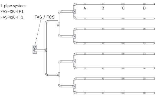
Quadruple U-pipe system for space protection
