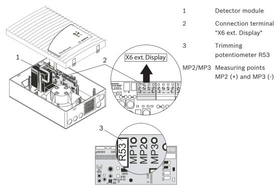
Air-pressure-dependent calibration of the airflow sensor
