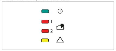
Figure 3.2: FAS-420-TP1/TP2, FCS-320-TP1/TP2 displays
