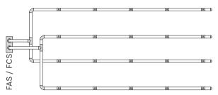
Pipe configurations for dual detector dependency
