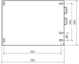
Figure 5.2: Bore distances of FCS-320 without mounting
