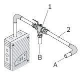
Components of manual blowing-out systems
