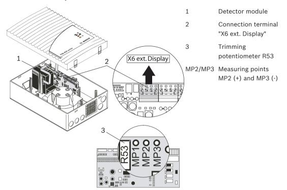
Air-pressure-dependent calibration of the airflow sensor
