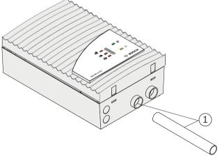
Connecting the aspiration pipe to the FCS-320 Aspirating Smoke Detector
