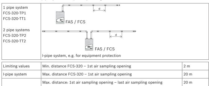
Max. number of air sampling openings (n) per pipe system
