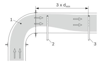
Direction change of the duct without air baffles
