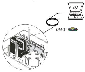
Figure 3.4: Diagnostic software for reading out unit status
