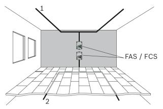
Principle of area monitoring with FCS-320 series Aspirating Smoke Detectors
