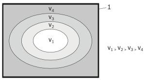
Speed distribution in an air-conditioning duct
