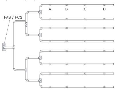
Quadruple U-pipe system for space protection
