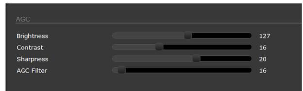
Experiment with different AGC parameters to find the settings that work best for the particular installation. Select **Save Settings** button at the bottom of the page to keep the settings after a power cycle or select the **Factory Defaults** button to return the settings to default values.
