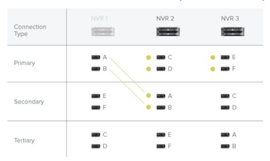
When NVR 3 fails, cameras E and F automatically connect to their Tertiary server, NVR 2.
