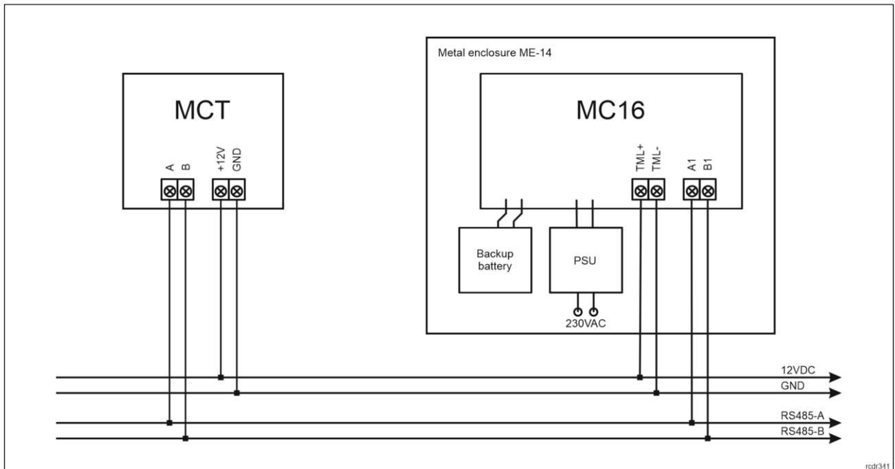
Fig. 1 MCT supply from MC16 access controller
