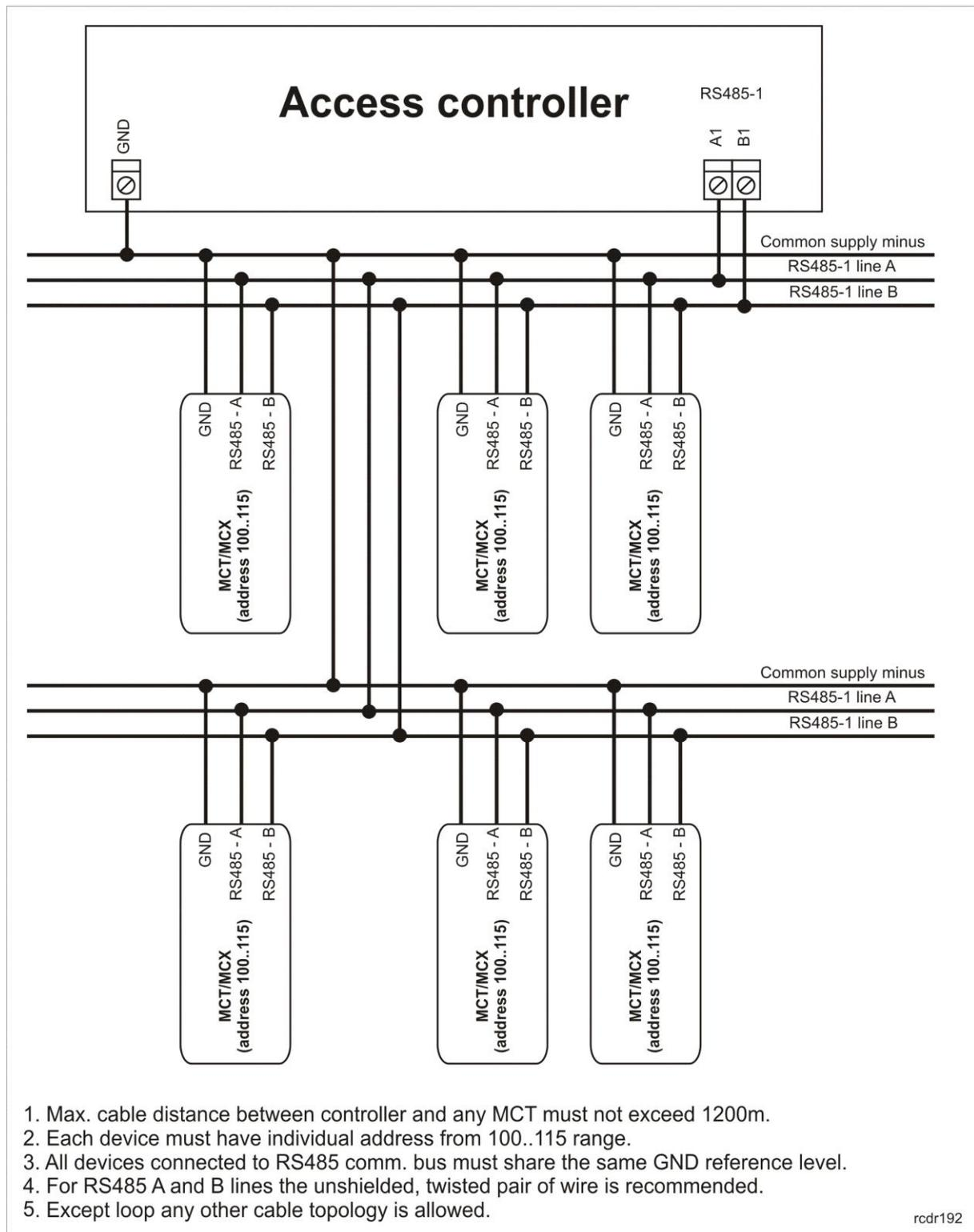
Fig. 5 Readers and modules connection to MC16.
