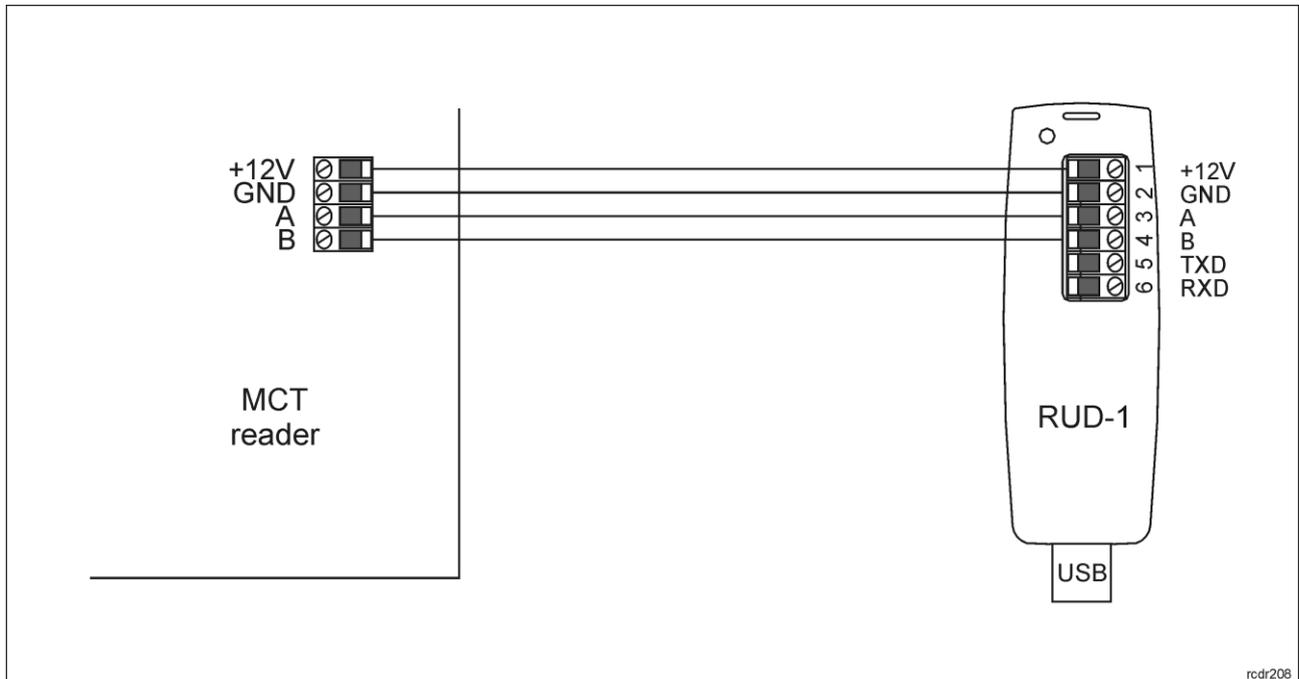
Fig. 7 Connection to RUD-1 interface (low level configuration).
