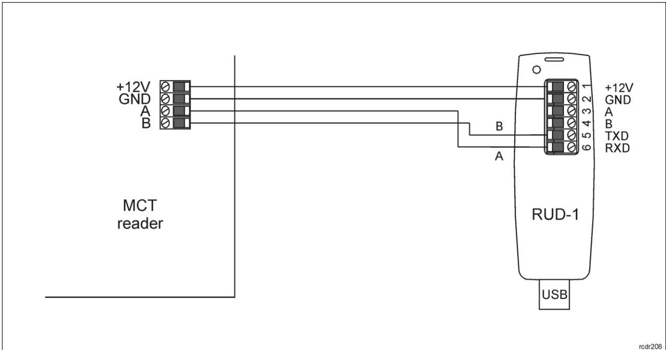
Fig. 8 Connection to RUD-1 interface (firmware update).
