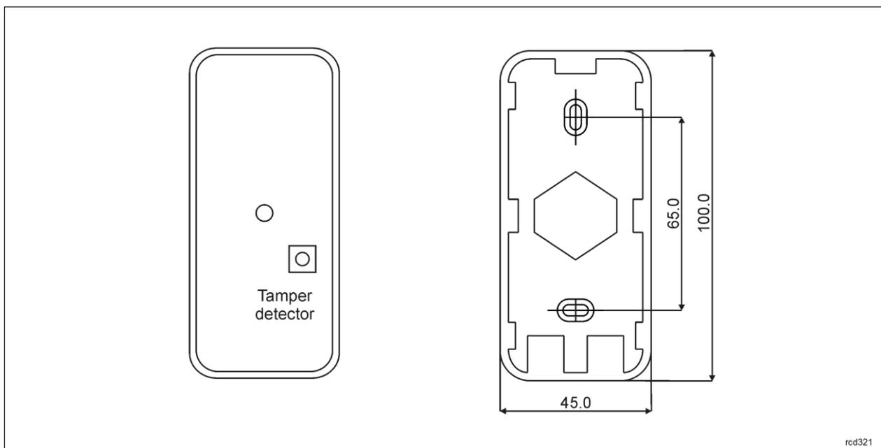
Fig. 5 Internal side of the front panel and back panel
