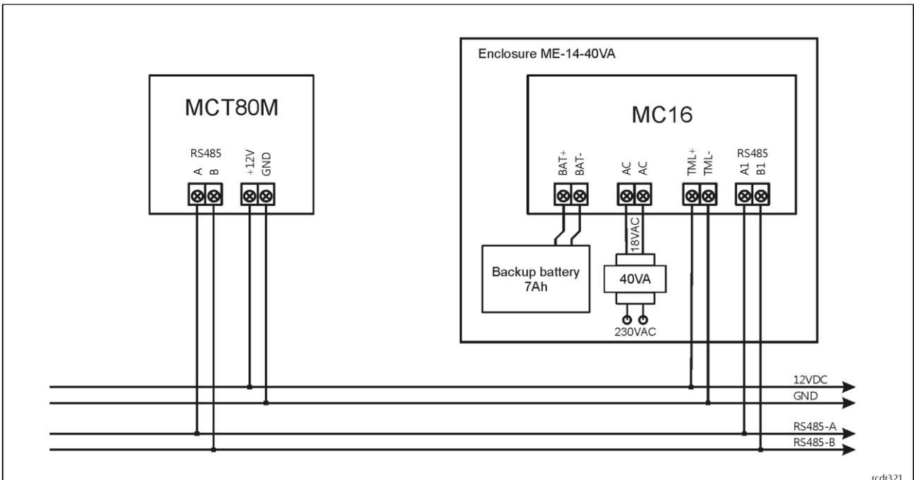
Fig. 2 MCT80M supply from MC16 access controller
