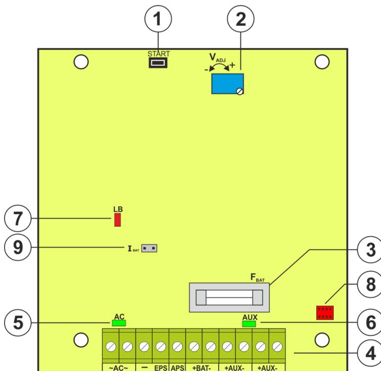
Fig. 2b. View of PCB board of 12V3A model
