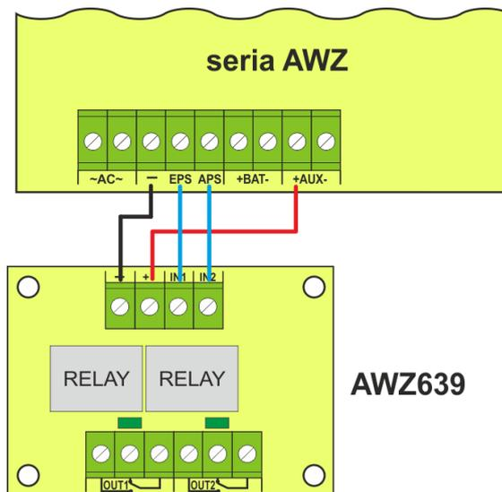
Fig. 5. The diagram of connecting the AWZ639 module.
