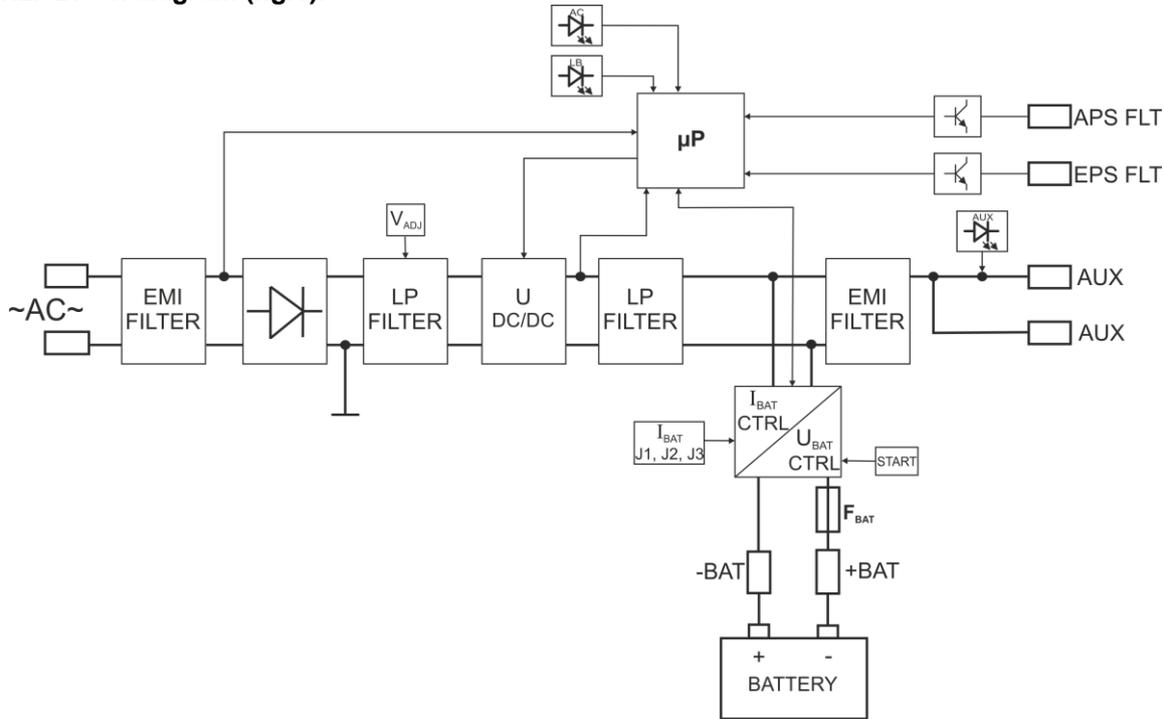
Fig.1. Block diagram of PSU.
