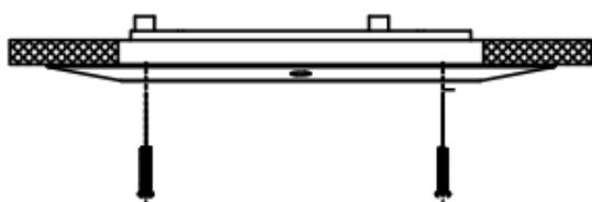
Figure 2-7 Install the In-Ceiling Mounting Bracket
