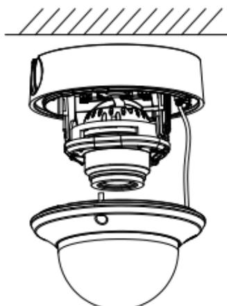
Figure 2-15 Fit the Black Liner Back
