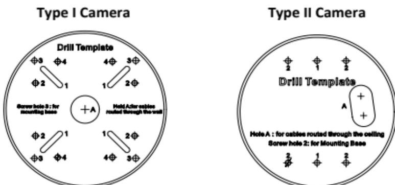
Figure 2-1 The Drill Template
