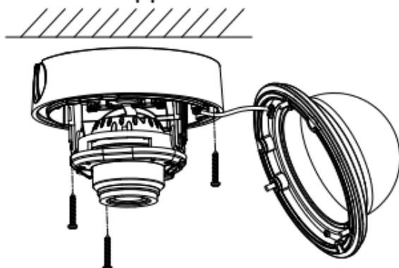
Figure 2-13 Attach the Back Box
