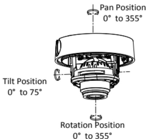
Figure 2-14 3-Axis Adjustment
