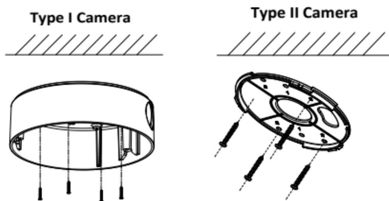
Figure 2-2 Attach the Back Box/Base Plate
