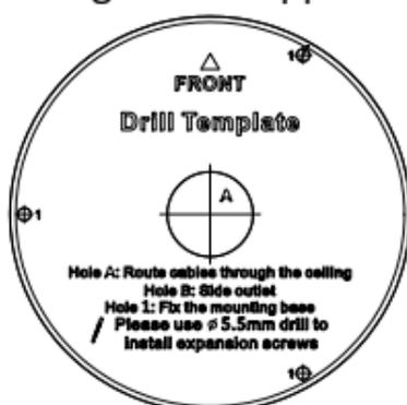
Figure 2-11 The Drill Template
