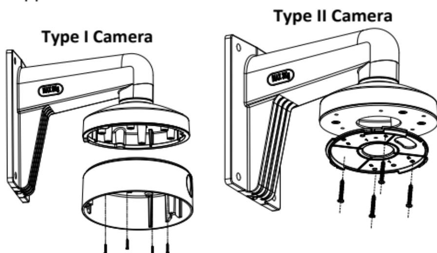
Figure 2-6 Attach the Base Plate to the Bracket
