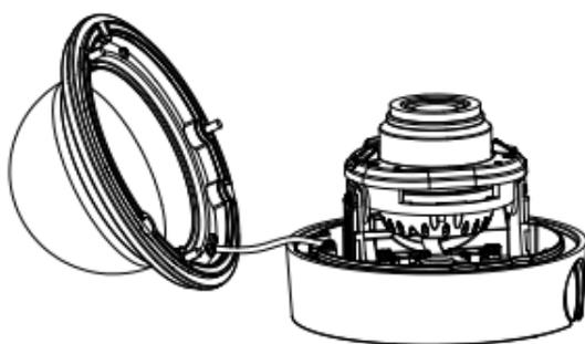
Figure 2-12 Remove the Bubble and the Black Liner
