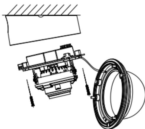
Figure 2-10 Fix the Camera to the Base
