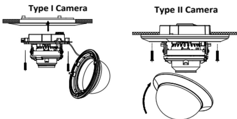
Figure 2-8 Fix the Camera to the Mount
