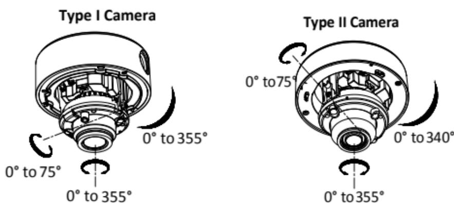
Figure 2-4 3-Axis Adjustment
