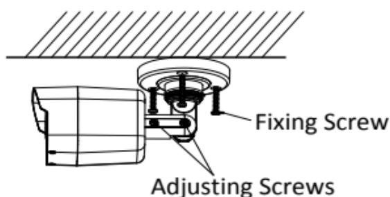
Figure 2-2 Fix the Camera to the Ceiling
