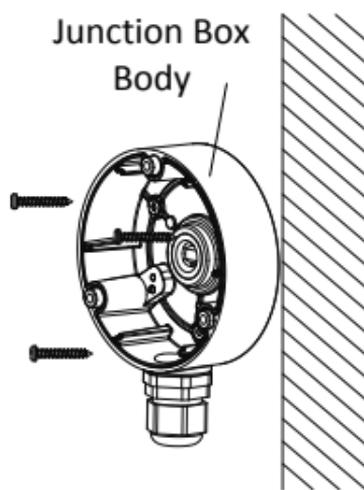
Figure 2-6 Fix the Junction Box to the Wall/Ceiling
