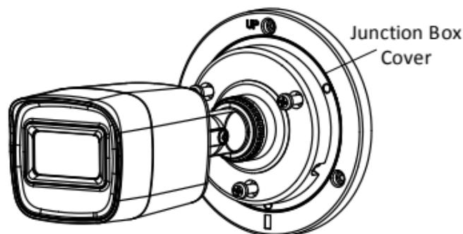
Figure 2-5 Fix the Camera on the Junction Box's Cover
