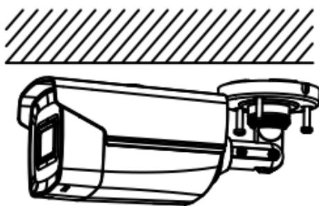
Figure 2-9 Fix the Camera to the Ceiling
