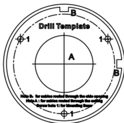
Figure 2-4 Drill Template of Junction Box
