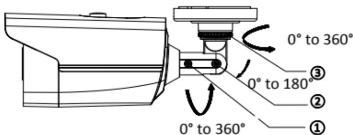
Figure 2-10 3-Axis Adjustment
