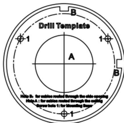
Figure 2-11 Drill Template of Junction Box
