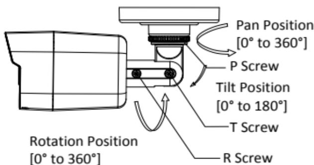
Figure 2-3 3-axis Adjustment
