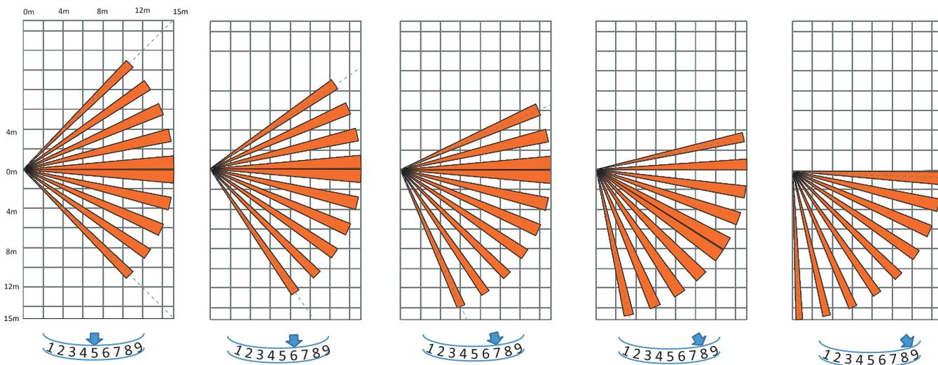
There are 5 scales in the vertical direction to adjust the detection distance.
