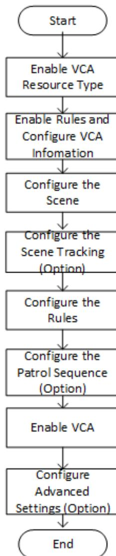
Figure 6-1 Flow Chart of Perimeter Protection Configuration
