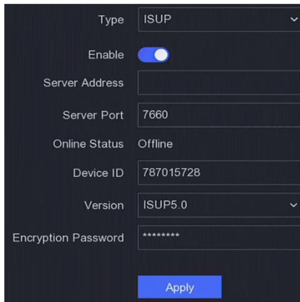
The screenshot shows a configuration panel for ISUP. The 'Type' dropdown menu is set to 'ISUP'. Below it, the 'Enable' toggle switch is turned on. The 'Server Address' field is empty. The 'Server Port' field is set to '7660'. The 'Online Status' is 'Offline'. The 'Device ID' field is set to '787015728'. The 'Version' dropdown menu is set to 'ISUP5.0'. The 'Encryption Password' field is filled with seven asterisks. An 'Apply' button is located at the bottom of the panel.
