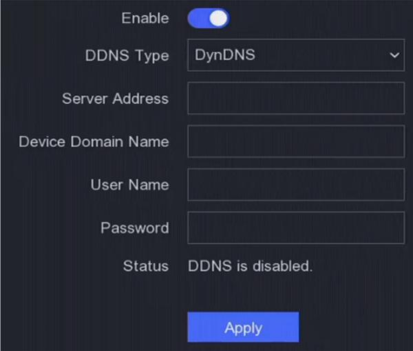
The screenshot shows a configuration panel for DDNS. At the top, there is an 'Enable' toggle switch which is turned on. Below it is a 'DDNS Type' dropdown menu currently showing 'DynDNS'. There are four text input fields: 'Server Address', 'Device Domain Name', 'User Name', and 'Password', all of which are currently empty. At the bottom of the panel, there is a 'Status' field displaying 'DDNS is disabled.' and a blue 'Apply' button.
