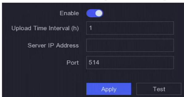
The screenshot shows a dark-themed configuration interface for Log Server Settings. At the top, there is an 'Enable' toggle switch which is turned on. Below it, there are three input fields: 'Upload Time Interval (h)' with the value '1', 'Server IP Address' which is empty, and 'Port' with the value '514'. At the bottom of the form, there are two buttons: a blue 'Apply' button and a grey 'Test' button.
