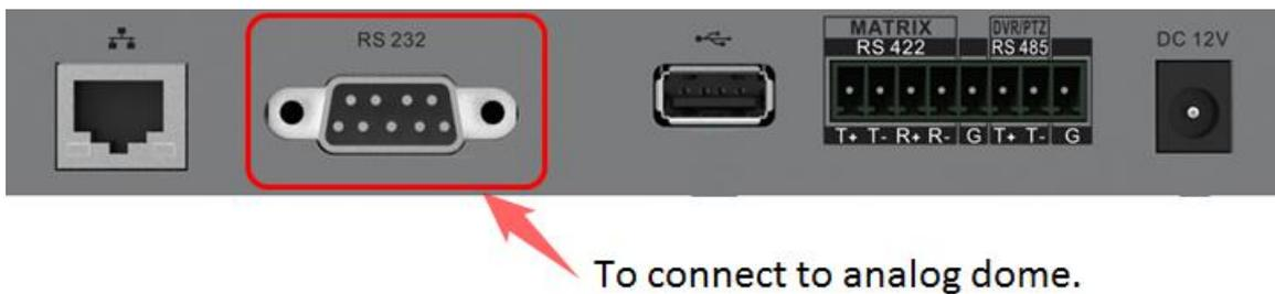
Figure 3-13 Analog Dome Connection
