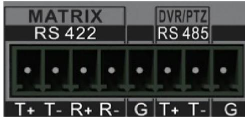
Figure 3-10 RS-485 Serial Port
