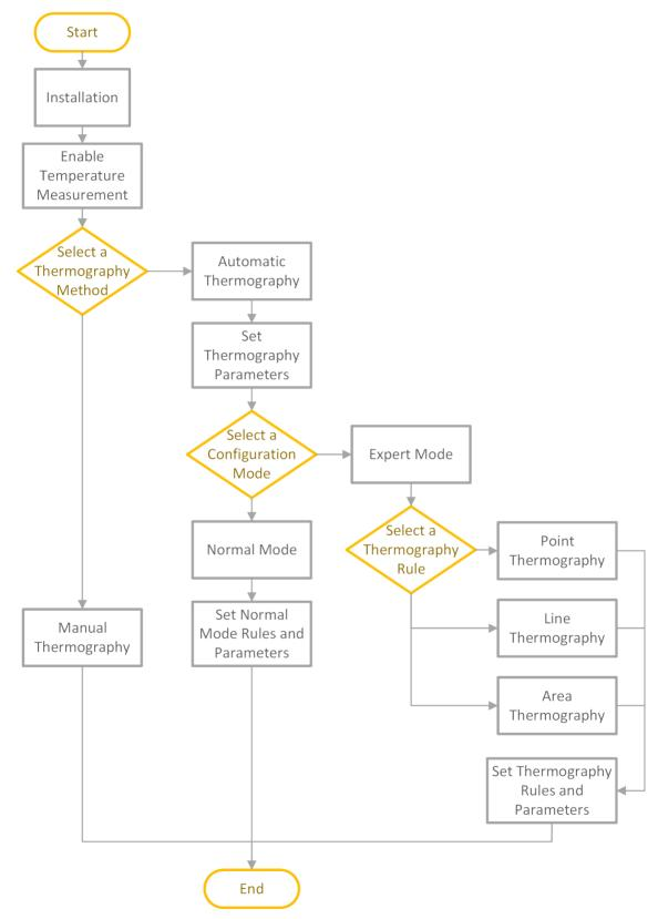
Figure 7-1 Thermography Configuration Flow Chart
