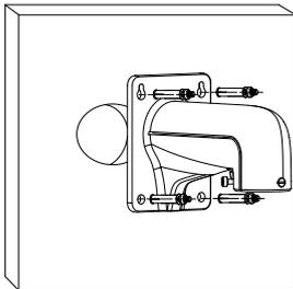
③ Tie the safety rope to hook and thread the cable
