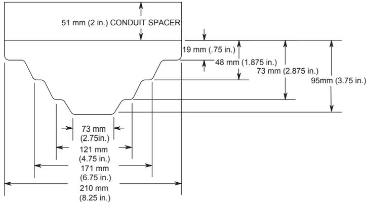
**DEPTH CHART OF THE POLYCARBONATE DETECTOR STOPPER**
