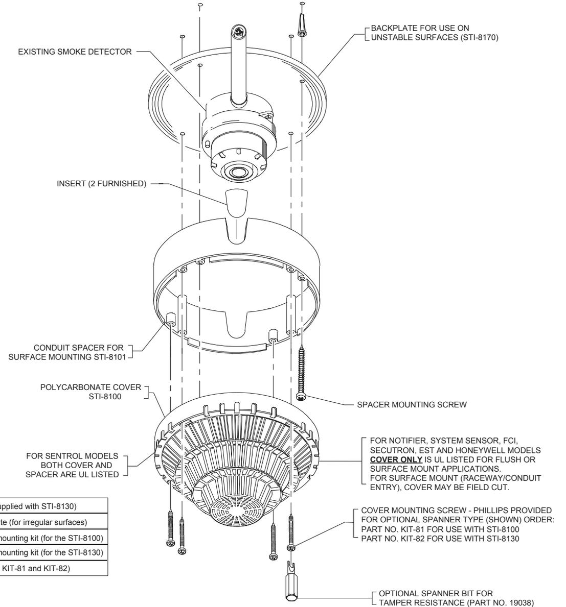
**INSTALLATION OF STI-8100 POLYCARBONATE DETECTOR GUARD**
