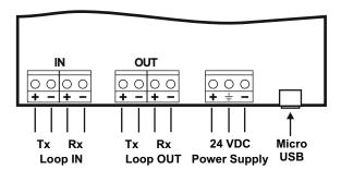
Loop IN - Connect the input line for communication Loop OUT - Connect the output line for communication Power Supply - Power supply for the repeater panel: - Use external 24VDC power supply unit; - Use the AUX output of the fire alarm panel.
