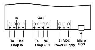
Loop IN - Connect the input line for communication Loop OUT - Connect the output line for communication Power Supply - Power supply for the repeater panel: - Use external 24VDC power supply unit; - Use the AUX output of the fire alarm panel. Micro USB - Micro USB input for programming and firmware update
