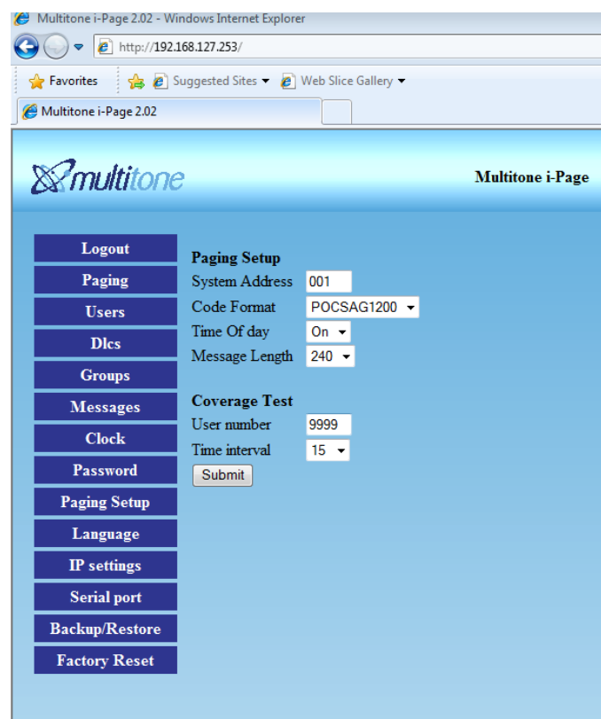
Figuur 25: Coverage test CQ-Net UMI Paging interface
