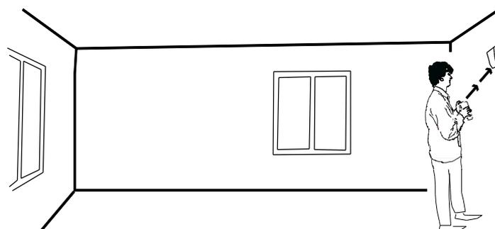
4. Go to the furthest distance (max. 9 m) of the glass to be protected and aim the speaker at the detector.
