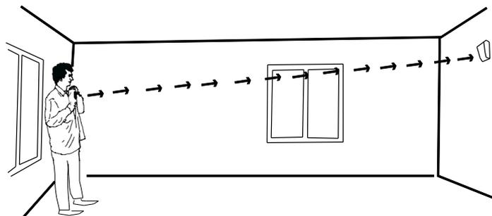
5. The DRC range calculated by the detector will be displayed as a number of pulses from 1 to 3.
